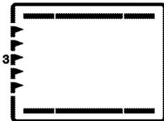
Food is heated simultaneously from the top and bottom. For example, it is suitable for cakes, pastries, or cakes and casseroles in baking moulds. Cook with one tray only.
