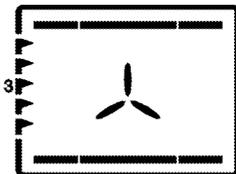
Hot air heated by the bottom and top heaters is evenly distributed throughout the oven rapidly by means of the fan. Cook with one tray.
