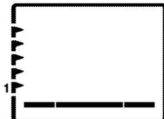
Only bottom heating is in operation. It is suitable for pizza and for subsequent browning of food from the bottom.
