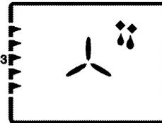
The oven is not heated. Only the fan (in the rear wall) is in operation. Suitable for thawing frozen granular food slowly at room temperature and cooling down the cooked food.
