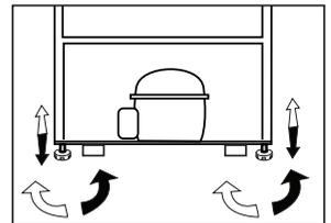
The backwall of the wooden cabinet must be left open completely to kitchen wall in order to allow sufficient air circulation to cool down the condenser unit for energy efficiency.
